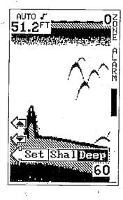
To adjust the zone alarm bar press the key adjacent to the up or down arrows. To adjust the top of the bar shallower or deeper, press the key adjacent to the Set Shal/Deep label until the word Shal is highlighted. To adjust the bottom of the zone alarm bar, press the key until the Deep label is highlighted. Now simply press the key adjacent to the up arrow to move the end of the bar up. Press the key adjacent to the down arrow to move it down.
